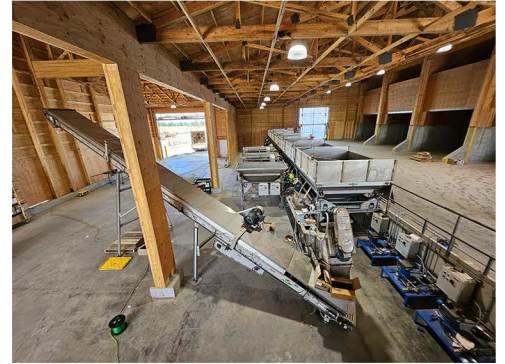
Featuring six 10-ton hoppers, three micro-hoppers, and a 10-ton material conditioner.
